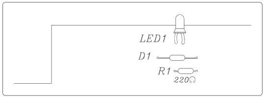
Figure 4.9 Layout of the LED
